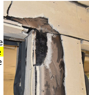
Beam-to-column connection tested at ATF Fire Research Lab.
